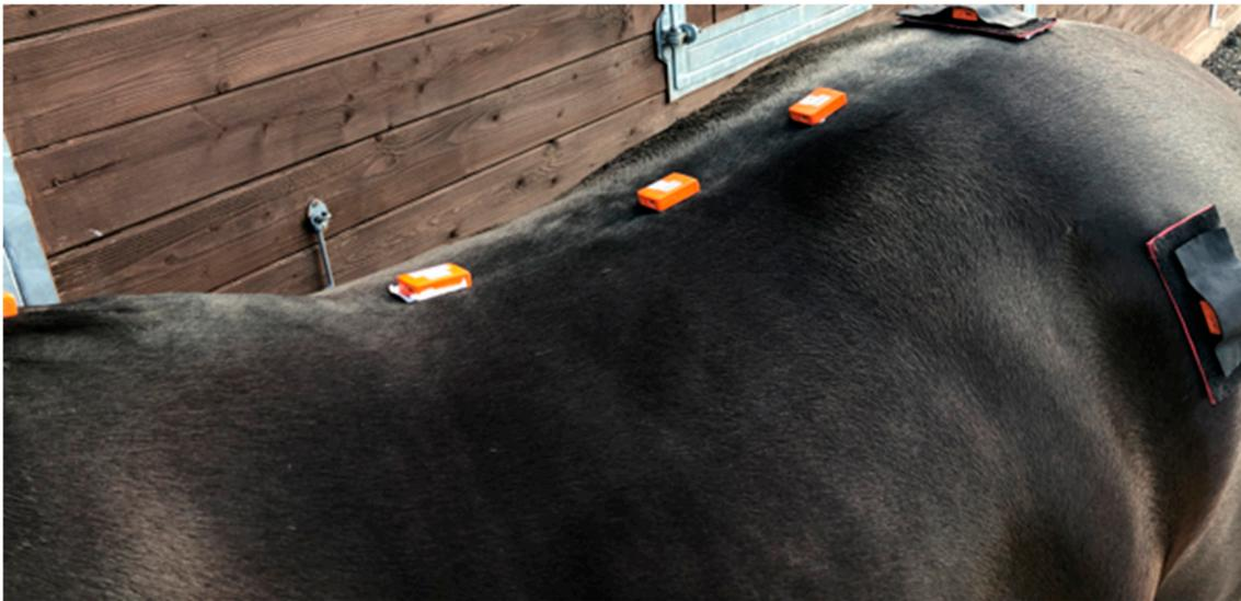
**Figure 2.** Inertial measurement unit (IMU) sensor locations along the thoracolumbar region. Sensors were glued on to the skin at T5, T13, T18, and L3. Sensor pouches were used for the tubera sacrale (TS) and left and right tuber coxae.
